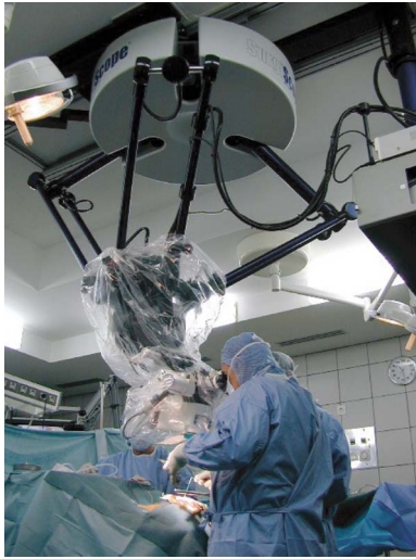
Fig. 1 A Delta robot used in the SurgiScope®, a robotized navigation tool holder designed for neurosurgery and developed by the Intelligent Surgical Instruments and Systems (ISIS) company
